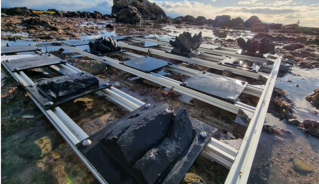
Figure 2: 3D models of mussel beds and rocky reef deployed on a frame at Fifeshire Rock, Nelson
